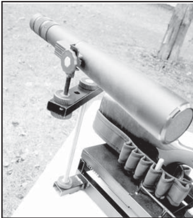
As An Extra Cost Option, A spotting scope mount is available (see replacement parts for details.) It consists of an M12 threaded rod which would fit in place of, and function as, one of the leveling screws, a horizontal support arm, that swivels and a scope mounting and bracket set. There are also 2 - M12 and 2 - M8 lock knobs to hold everything in place.
